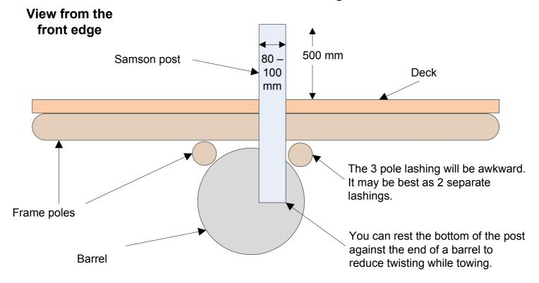
The Samson post is used for towing a raft.
